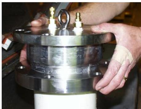
Slide clamp ring housing up over the inserts and bolt on. Follow same bolt procedure as the bottom assembly.
