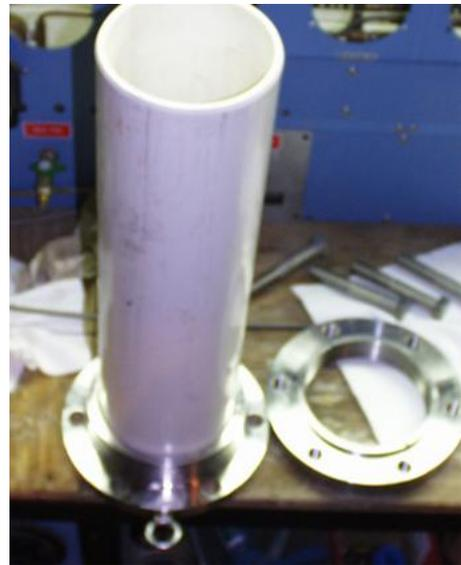
Inserting pipe into bottom endcap assembly
